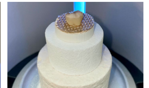
The crown is placed on top of the CEREC SpeedFire honeycomb tray with a firing pad. It must be centered on the pad. The construction is then placed in CEREC SpeedFire.
