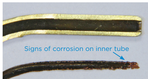
CLOSE-UP OF INNER AND OUTER METAL TUBES
